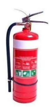
Power Based Fire Extinguishers: - Supply and fixing of ABC stored pressure squeeze grip type fire extinguishers, 4 kg capacity, IS:15683: 2006, filled with ABC Mono Ammonium Phosphate base powder-90 complete with discharge hose and wall mounting bracket, 2mm Mild Steel, EPDM Rubbers, Pressure Guage, which work effectively on all class of fires (A,B,C & Electrical fires)
